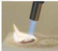
Fire metal clay quickly with a hand-held torch.
