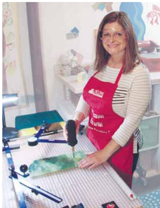
The foam cushioned, weighted handle eliminates the strain of grasping a cutter.
