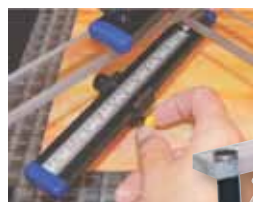
Use ruler to adjust cutting head for precise circles. Just press down on the knob to score, no heavy pressure is needed.
