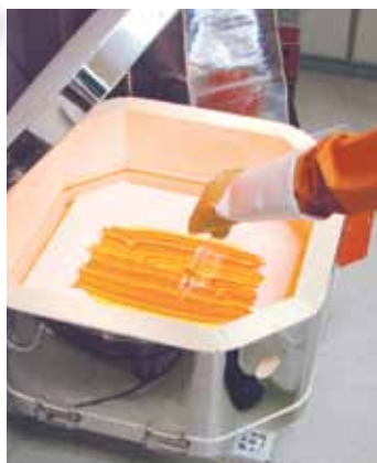
Rake shown combing molten glass in kiln.
